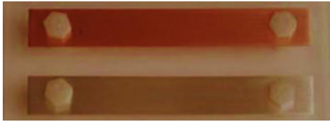
FIGURE 16.3 Photo of the CCC. The standard method for analyzing corrosion coupon is called cathodic/electrolytic reduction. The thickness of the corrosion film is determined by a laboratory analysis. The results of the report included photograph of returned coupon strips, ISA Environmental Classification, and film thickness/30 days.
