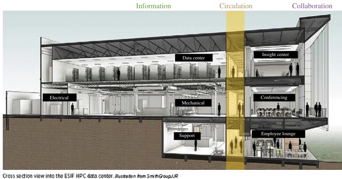
FIGURE 1.7 ESIF's high-performance computing data center—innovative cooling design with PUE at 1.06 [33].
